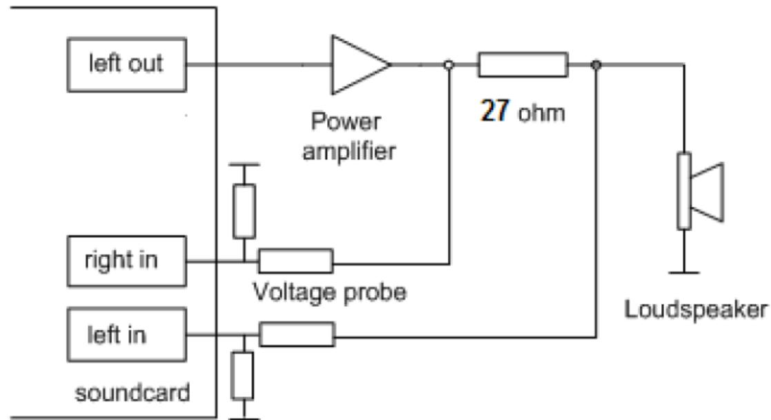
**Figure 3.2** General measurement setup for loudspeaker impedance measurements
