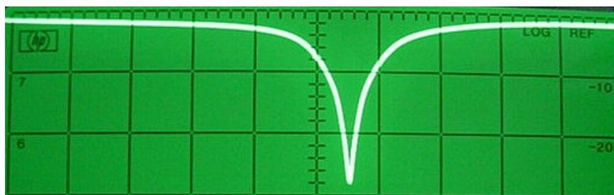
This shows RF return loss from 88 to 108 MHz with the XDR-F1HD tuned to 98 MHz. The dip is 1 MHz high. Its frequency does not monotonically increase with tuned frequency, backstepping at 90.2, 92.8, 95.4, 98.0, 101.4,
