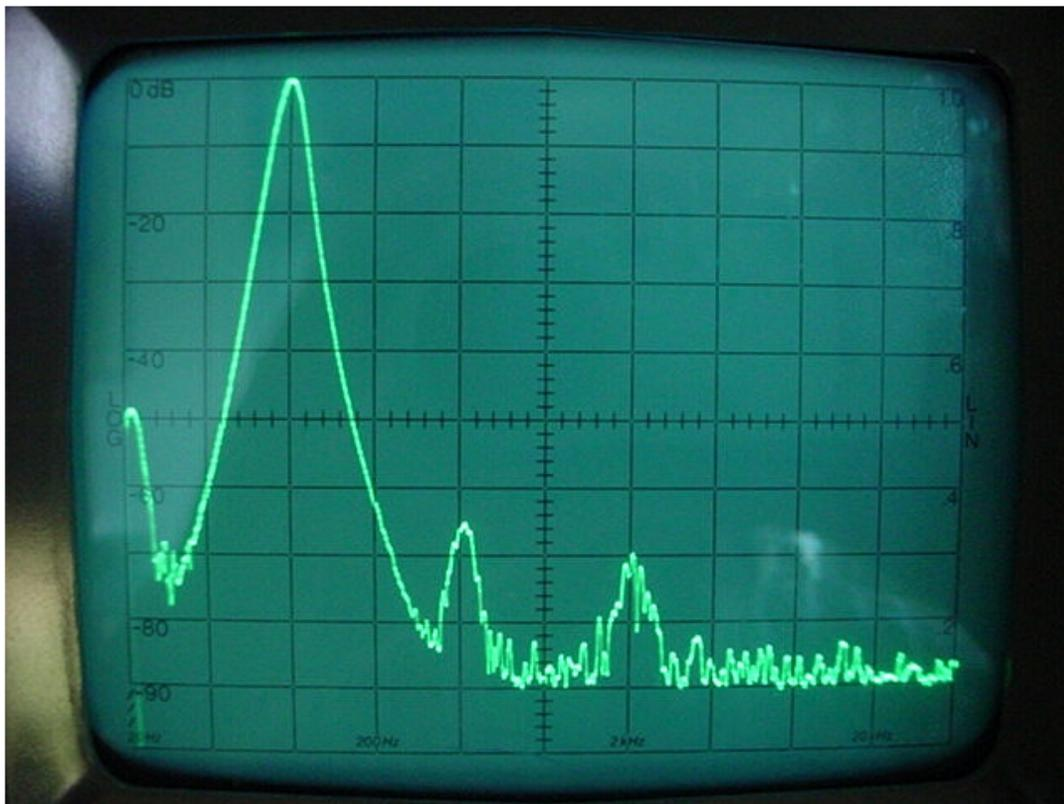
This is the distortion spectrum for 1-kHz, single-channel, stereo modulation deviated 75 kHz with 9% pilot.
