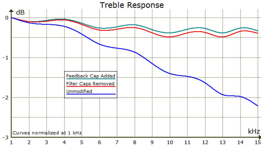
Each D/A feeds a ferrite bead and shunt capacitor within the tuner module. The module drives two-section, passive, RC lowpass filters on the motherboard. The filters suppress low-level ultrasonic noise that extends to a few MHz, but they also cause the frequency response to droop within the audio passband, as shown by the blue curve. The ultrasonic noise is due to D/A noise shaping that maximizes S/N within the audio passband.
