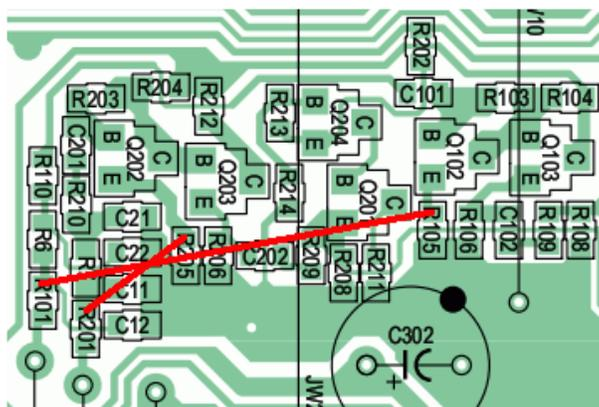
The second way to correct the droop is to add a feedback capacitor from the audio stage to the filter. The green curve shows the response. You may find this method easier than unsoldering surface-mount parts. With the PCB oriented as above, connect 0.01  $\mu\text{F}$  between the upper ends of R101 and R105. Add another between R201 and R205 for the other channel. The capacitors must be very thin for the PCB to properly seat.
