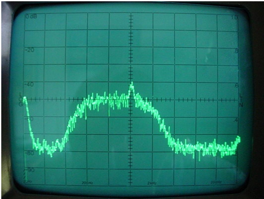
This is the left-channel response. The noise has a pronounced narrowband sound quality. The tone frequency determines the position and bandwidth of the noise hump. Multiple tones cause multiple humps, and a complex signal spectrum acquires a filter adapted to its specific shape. Exploration with a sine wave reveals that the noise reduction algorithm uses a discrete frequency-domain filter bank rather than a continuous time-domain technique. I counted 17 filter passbands.
