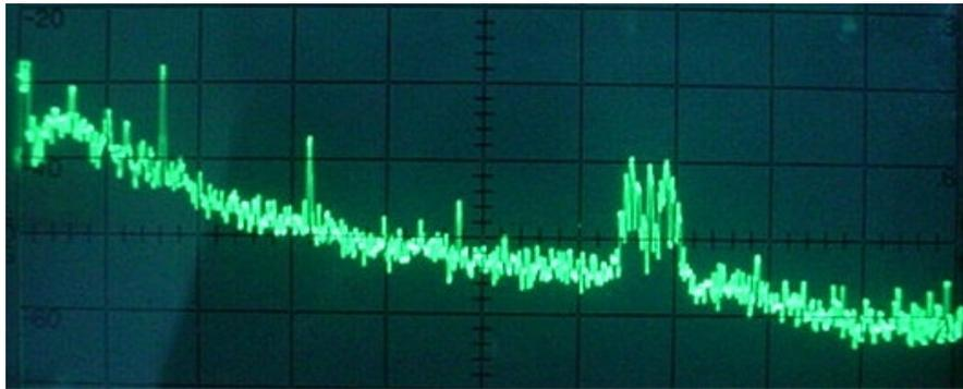
For a strong unmodulated test signal, I could hear a faint whine in the background noise with the volume turned way up. This image shows the audio spectrum to 20 kHz using a 30-Hz analysis-filter bandwidth and postdetection smoothing. I think I was hearing the pip just above 3 kHz. Close examination reveals it to be at 3125 Hz and 78 dB below 100%, 1-kHz modulation. I have yet to hear the whine in a broadcast signal. (The thicket at -90 dB between 13 and 14 kHz was absent in a second tuner.)
