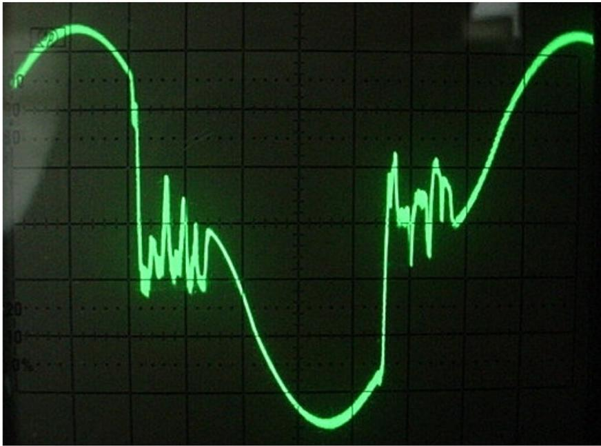
I observed these glitches for a 100%-modulated, 20-Hz, monophonic test signal. The waveform reminds me of a PLL detector losing lock, but I don't know the actual cause.
