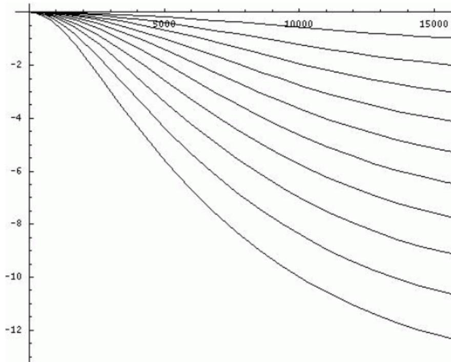
In addition to the adaptive noise reduction on L-R, the XDR-F1HD gradually applies a high-cut noise filter to L and R when the RF level drops below 26.5 dBf. The filter progressively affects lower frequencies as the signal level falls, as shown above. It is similar to the high-cut filter in the HDT-1X.
