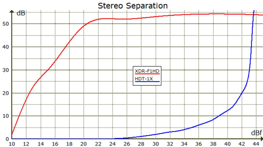
This compares 1-kHz stereo separation for the XDR-F1HD and HDT-1X as a function of signal level. The Sangean protects the listener from noise by rapidly blending the channels when S/N drops below 56 dB. The Sony's adaptive noise reduction takes care of the problem for a further 20+ dB drop in signal level without degrading channel separation.
