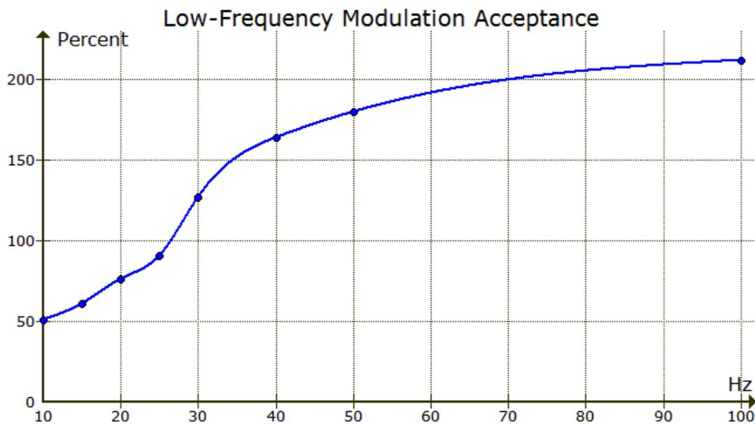
This shows the maximum glitch-free modulation level at low frequencies. I've never identified one of these glitches on a broadcast signal.
