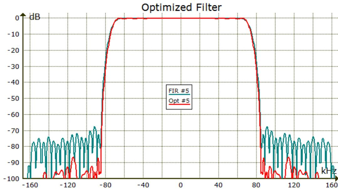
With an I<sup>2</sup>C bus controller it is possible to alter the SAF7730 filter coefficients. This plot compares FIR filter #5 with an [optimized filter](#). However, reciprocal mixing of local oscillator phase noise evidently limits any stopband improvement (see the VCO spectrum below). Konrad Kosmatka could not hear a difference between these two filters when tuning broadcast signals.
