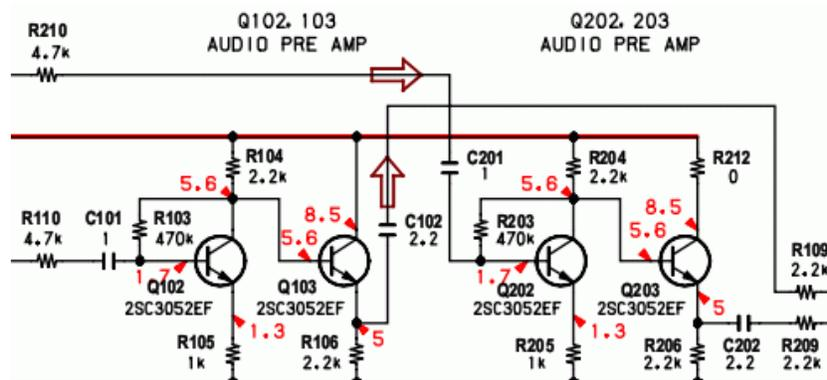
In addition to clipping, the bipolar amplifiers in my tuner degraded second-harmonic distortion 10 dB. To replace them, see **Treble Correction**.
