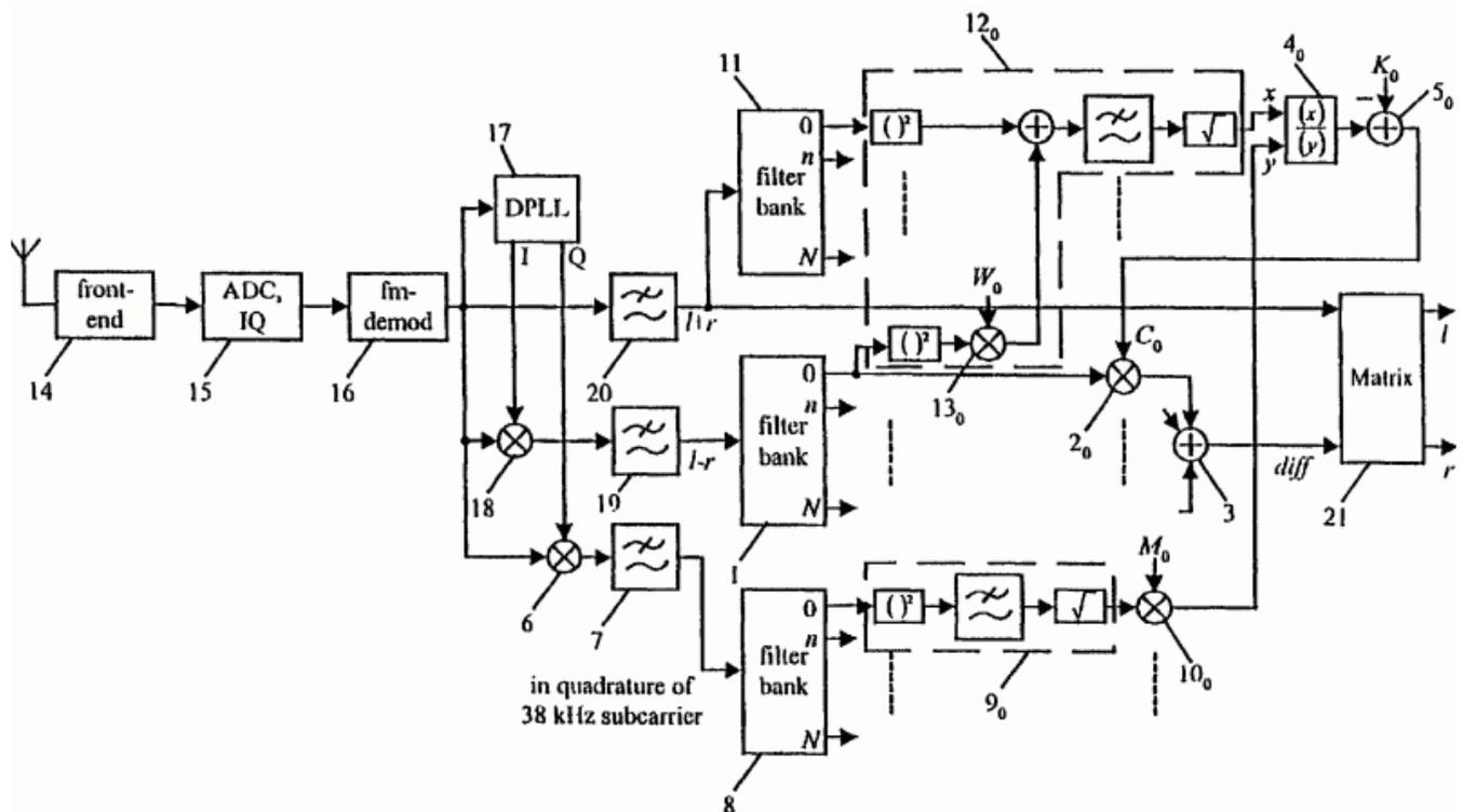
Adaptive noise reduction affects only the noisy L-R stereo subchannel. The algorithm attenuates filter bank outputs according to critical-band auditory masking criteria. U.S. patent [7,110,549](#) describes the method, while [7,292,694](#) refines it. The quadrature L-R signal [normally](#) provides a robust estimate of the background noise level in each bank.
