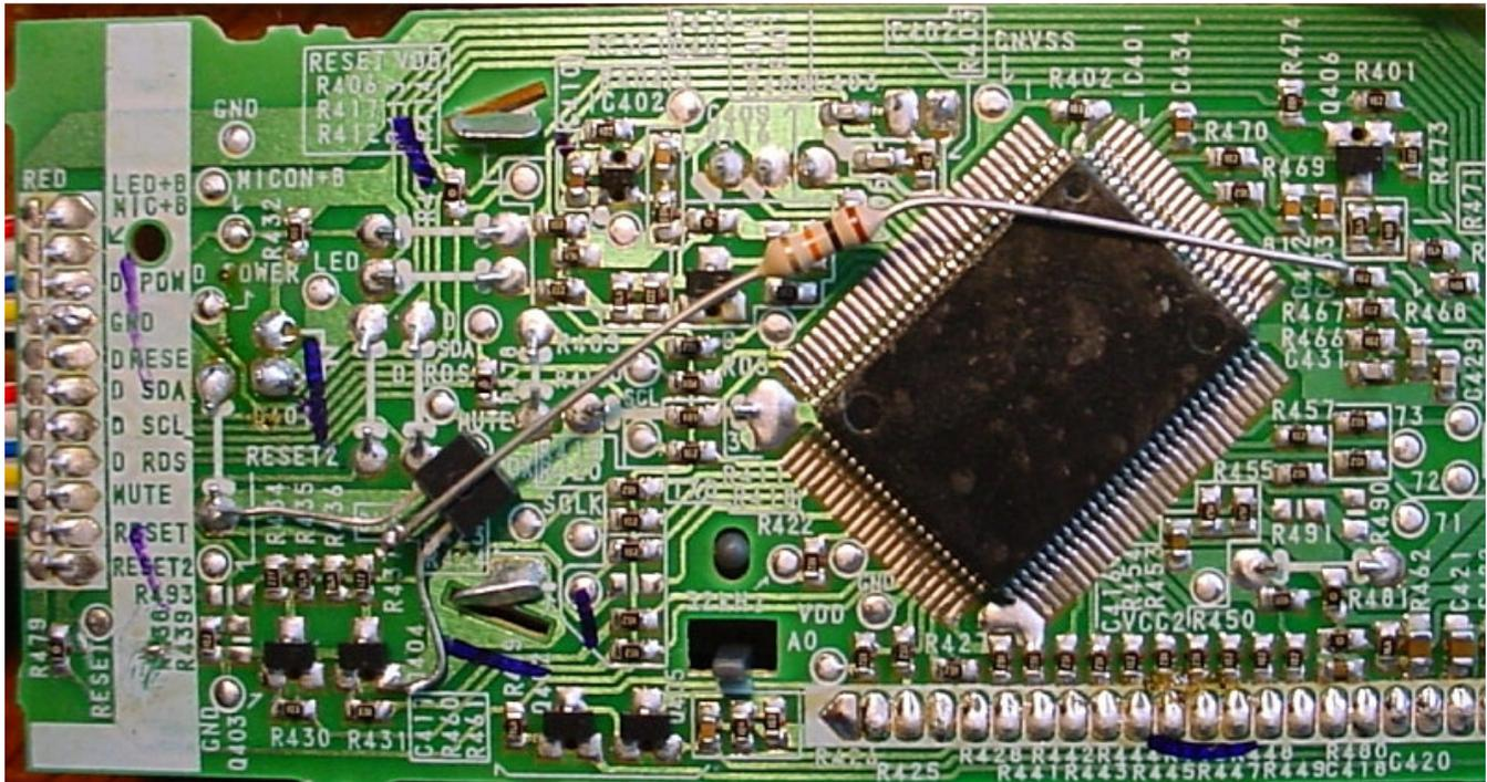
Even when dimmed, the LCD may be too bright in a bedroom at night. Cutting a trace on the controller board and installing a transistor and resistor will disable the backlight in standby.
