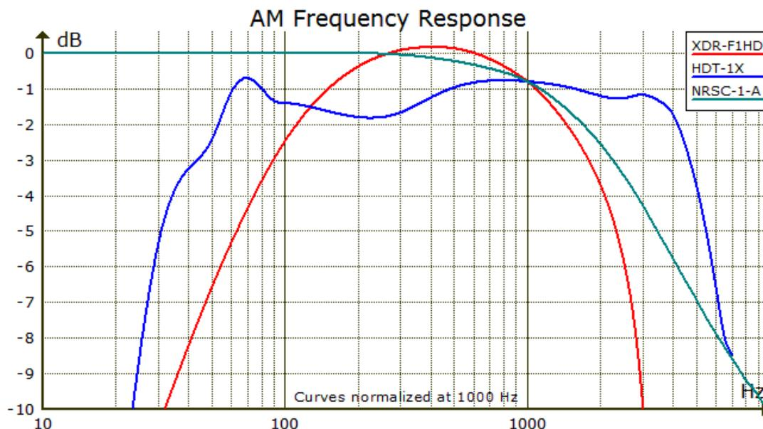
This compares the frequency response of the XDR-F1HD and HDT-1X with the [NRSC-1-B](#) AM deemphasis standard. The error is easily audible for both tuners. I wondered whether the Sony's bass roll-off might be intended to comply with the old tonal balance rule for AM radios, which states that the product of the low- and high-frequency limits in cps should be about 500,000. The bass response actually extends more than twice as far as the rule stipulates.
