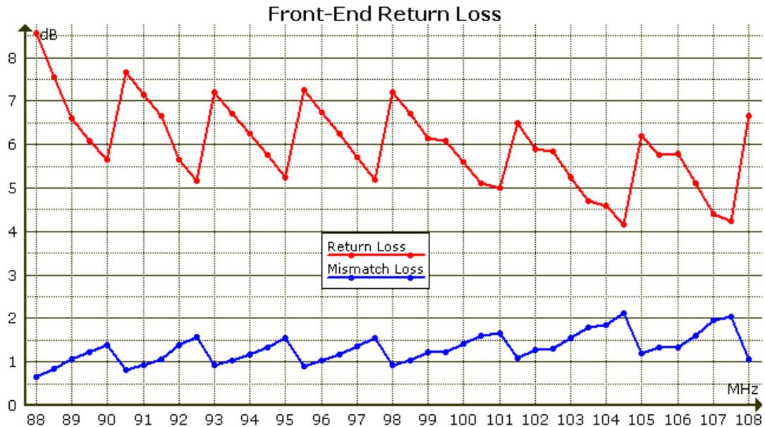
This is tuned-frequency return loss and the resulting mismatch loss. Mismatch loss directly increases tuner noise figure and degrades sensitivity. Add an RF preamp to [swamp](#) it or see **Alignment** to retune the front-end.
