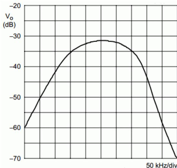
A 180-kHz Murata ceramic with this response acts as a roofing and antialias filter for the digital IF.
