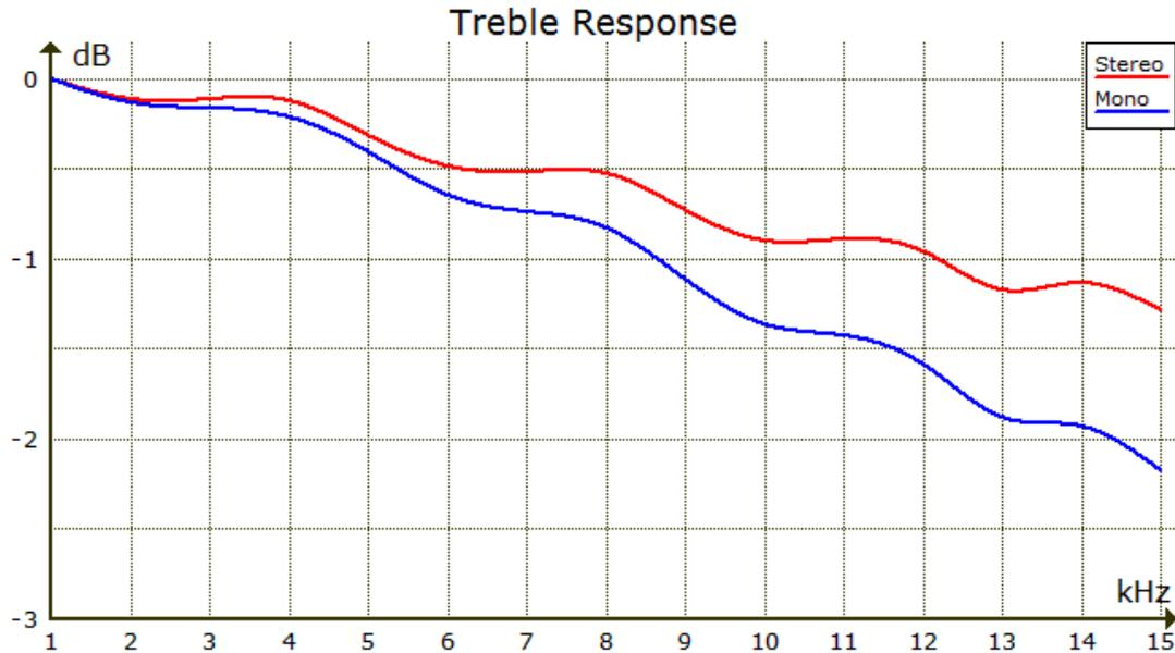
This is the left-channel treble response with an IEEE load ( $100\text{k}\Omega \parallel 1000\text{ pF}$ ). I don't know why the curves differ or why they are wavy. To flatten the droop, see **Treble Correction**.
