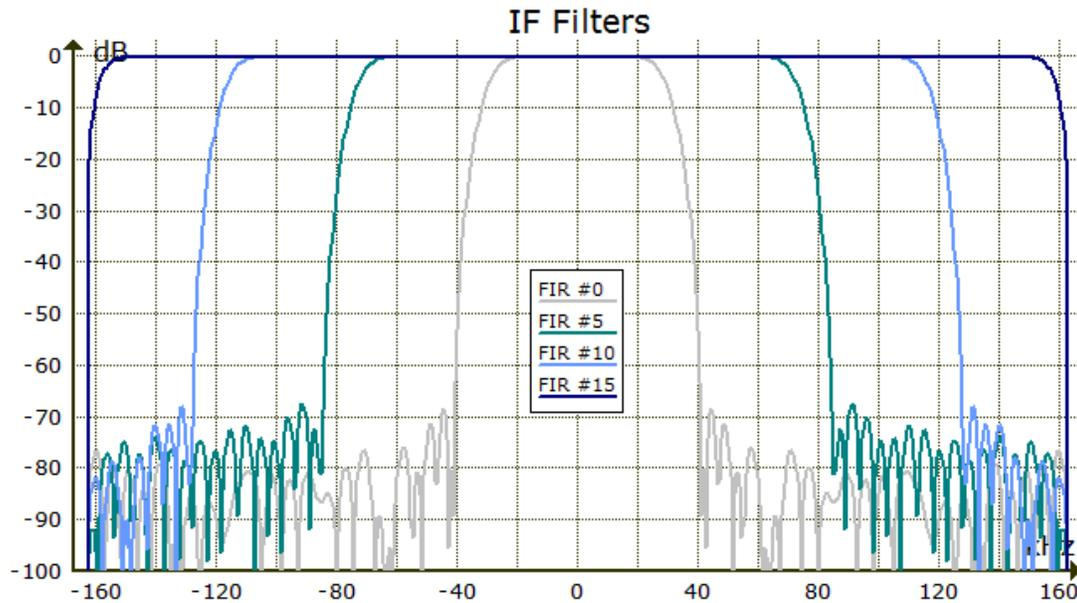
The SAF7730 provides 16 IF filter bandwidths. It automatically sets the bandwidth based on interference and modulation level. The 64-tap FIR filters use 16-bit coefficients. This graph shows the response of four of the stock filters, from narrowest to widest. The narrowest filters lower the FM threshold when the modulation level is low.
