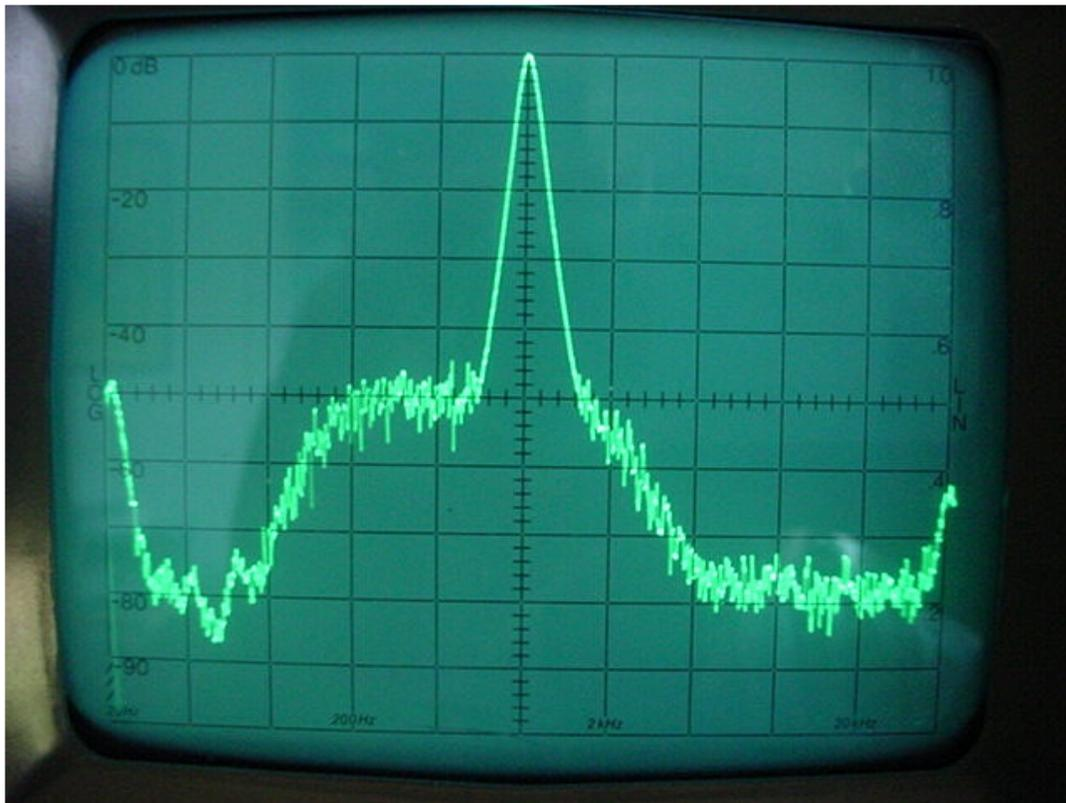
This shows the audio spectrum for a 1-kHz right-channel tone at an RF level of 22 dBf. The horizontal scale is 200 Hz/div and vertical is 10 dB/div. The shape of the adaptive filter is evident from the noise hump.
