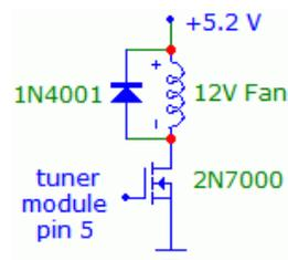
A tiny fan mounted inside the tuner should greatly lower its temperature. Many 12V fans become inaudible when operated at a lower voltage. Try the unregulated +5.2V, switching the fan and a back-biased diode with a transistor driven by the 8.5V.
