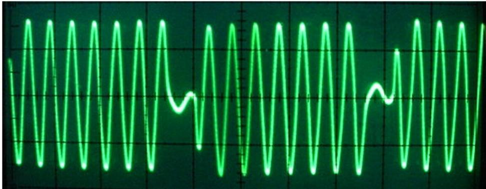
The XDR-F1HD has an automatic noise blanker. This shows it blanking lamp dimmer pulses in sinewave modulation (2 ms/div). Blanked audio sounded somewhat rough, with 1.2-ms waveform segments erased every 8.3 ms. Still, with strong pulse interference the audio sounds much better blanked than not.
