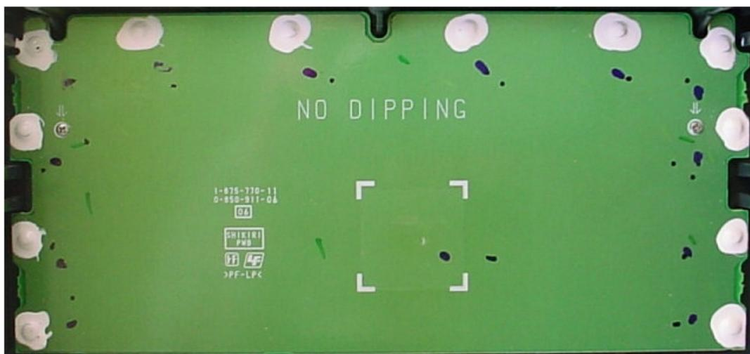
On the underside of the top cover is a curious bare PC board attached with screws and adhesive. A small square of plastic film insulates contact with the tuner module. The board is marked SHIKIRI PWB. *Shikiri* means partition, division, boundary, or compartment. It is also the ritual where sumo wrestlers down on their fists glare fiercely at each other before a match begins. Surely one of these definitions provides insight.
