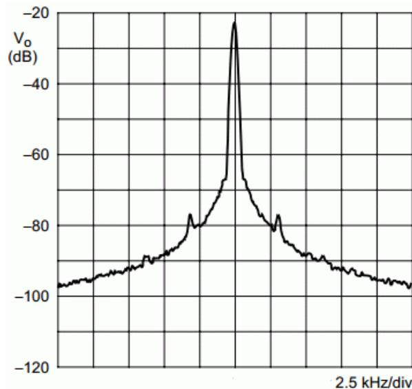
This is the spectrum of the TEF6730 voltage-controlled oscillator. The two small sideband peaks have the right offset and level to account for the whine. The vertical scale is dBc/Hz.
