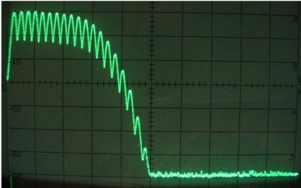
This is the audio output spectrum for a test signal consisting of NRSC-preemphasized tones spaced 250 Hz. The horizontal scale is 1 kHz/div and vertical is 10 dB/div. The plot confirms my listening impression that the XDR-F1HD severely rolls off the AM high-end. The response is down 24 dB at 4 kHz.
