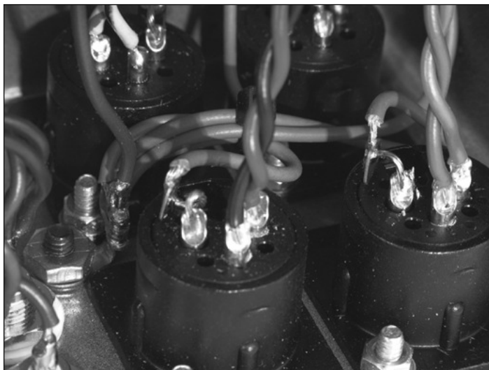
PHOTO 14: Pin 1 grounding.
